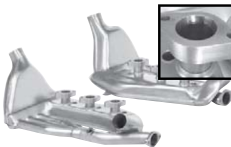
91.936SSI (1623105310) Heat exchanger set, stainless steel, left/right Europe/USA: Porsche® 911, 3.6 (Conversion), installed in 65-89 chassis. Requires further modification to install.
