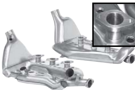
91.913SSI (1623105010) Heat exchanger set, stainless steel, left/right Europe: Porsche® 911, 2.2-2.4, 72-74 (inj.) Porsche® 911 Carrera, 2.7, 74-76 USA: Porsche® 911, 2.2-2.4, 72-74 (inj.)
