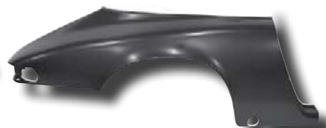
591052 (1680400480) right (OE 911.503.062.43) Quarter panel Targa, 69-73 Painted spcc steel
