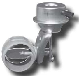
EQ253096 (1619900502) Exhaust gas flap, Pierburg no. 7.28153.18.0 Height: 128.9 mm, Width: 124 mm Flap Ø: 52 mm, Inner Ø: 55.6 mm Outer Ø: 56 mm, Connection angle: 233° Tube angle: 90°, Zero position: open
