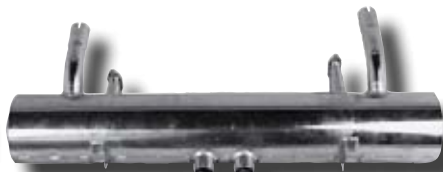
92.311S (1620606700) (OE 616.111.010.05S) Rear exhaust Polished stainless steel 304/4301 912 export USA
