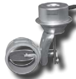
EQ253095 (1619900402) Exhaust gas flap, Pierburg no. 7.28153.16.0 Height: 128.9 mm, Width: 124 mm Flap Ø: 52 mm, Inner Ø: 55.6 mm Outer Ø: 56 mm, Connection angle: 153° Tube angle: 90°, Zero position: open
